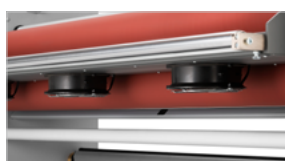
Vacuum feed in table complete with fans for thin papers (optional)
