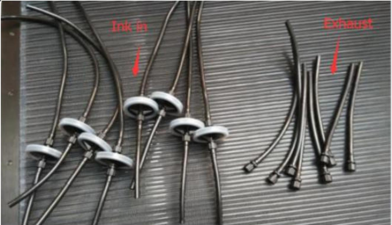
3 Check the filter and the inlet tube, make sure the lower tube is thicker than upper tube, then connect the big connector. Also connect the outlet tube with the small connectors.
