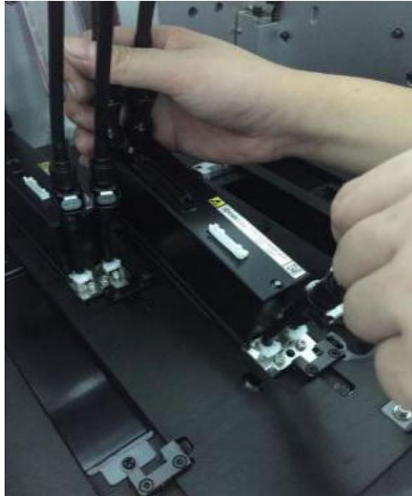
11 Discharge the protective fluid of the head
