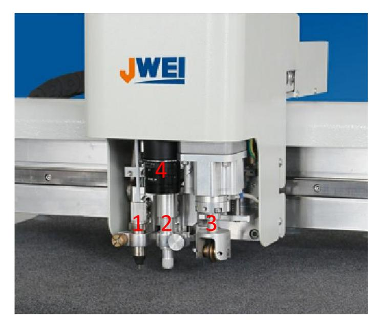
Cutting tool(Passive) /Plotting Pen
